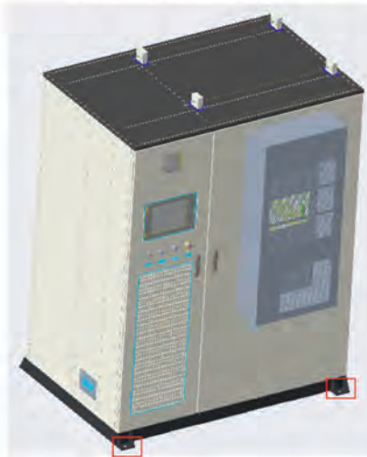
Figure 3-4 Securing the Energy Storage System
