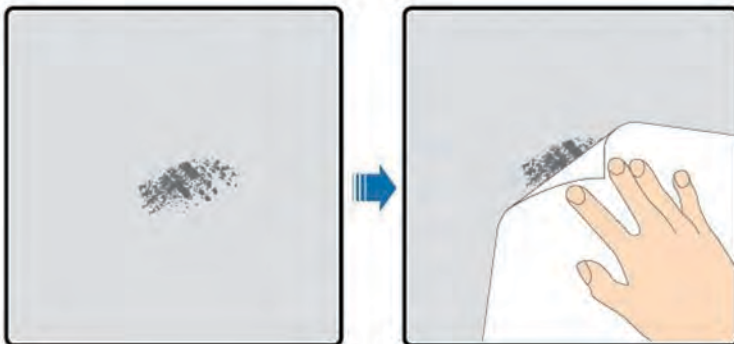
Figure 4: Sanding the Coating Damage with Fine Sandpaper
